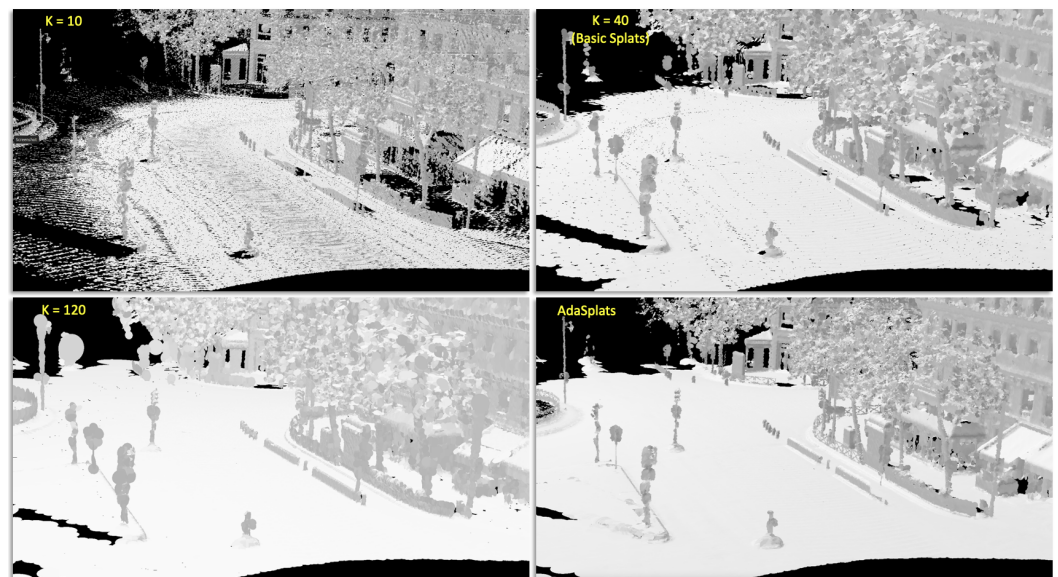
Figure 7. Rendering results on different choices of \mathcal{K} -nn on PC3D-Paris dataset. A small \mathcal{K} (e.g., 10 or 20) results in holes on the surface and ground groups while also resulting in a better approximation on the non-surface and linear groups. A large \mathcal{K} (40 to 120) results in a hole-free approximation of the surface and ground semantic groups while creating artifacts on small structures belonging to the linear and surface groups.
