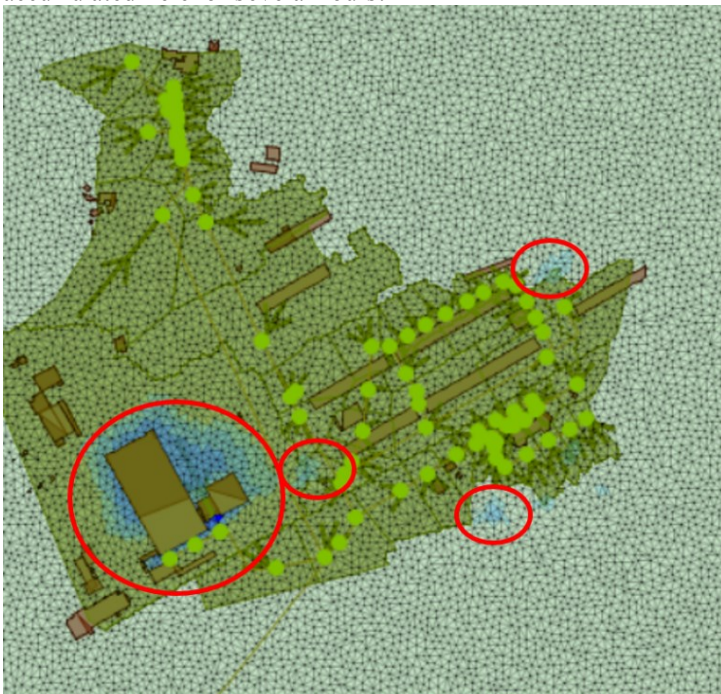
Figure 7. Maximum water depths modelled with 1D/2D model for the 100 years return period event
