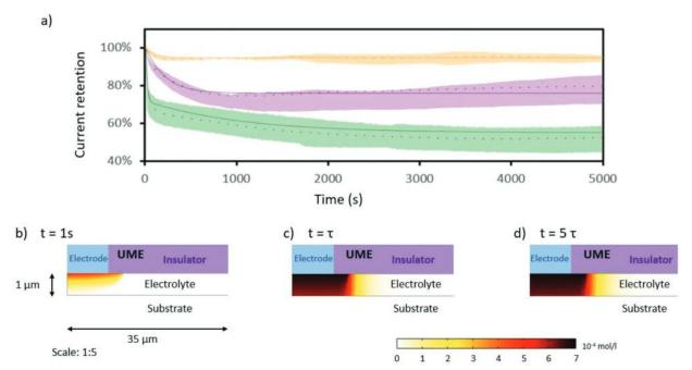
Figure 7. Fast local degradation of nanocomposite electrodes. a) Experimental values (dots lines) and simulations (plain lines) of SiWafer (purple), SiNWs (orange), and SiNTrs (green). Tolerance is expressed by the shade around the dots. b—d) Diffusion layer of [Ru(NH3)6]2+ at different characteristic times of degradation. The color shows the diffusion layer of oxidated redox shuttle between the tip of the UME (blue) and the electrode.
