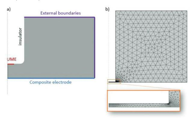
Figure 2. Schematic representation of the SECM experiment. a) Simple model with the electrolyte domain represented in grey, the UME surface in red, the composite electrode surface in blue, the insulator around the UME in black, the external boundaries in purple, and the symmetry axe as a dashed grey line. b) On scale model with the applied mesh. A magnified view of the electrolyte under the UME is presented in the orange rectangle. The tip-electrode distance is here 1  $\mu$ m.
