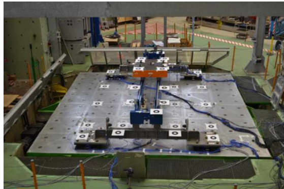
Fig. 2 – Overhead crane bridge mock up put on the AZALEE shaking table.
