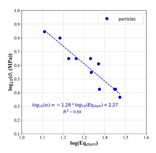
Figure 5: log plot of evolution of true stress at the decohesion onset ( $\sigma_i$ ) with the  $Eq_{diam}$  of the metallic particle (S 4.3 material). Dotted line for the linear curve fitting.
