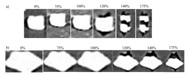
Figure A1: Damage evolution in a material containing 3% volume fraction of ZnO. A) at 120% nominal strain, there is a decohesion at the poles followed by fracture of ZnO at 140% nominal strain. B) decohesion at the poles of ZnO inclusion at 120% nominal strain, without subsequent fracture of the inclusion.
