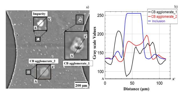
Figure 2: a) slice view of ROI of an S\_9.0 test sample. Zoomed areas correspond to a metallic particle and two CB<sub>aggl</sub>. The grey scale intensity values across the lines drawn through these defects are plotted in b).
