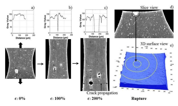
Figure A4: Crack initiation mechanism for S\_4.3
