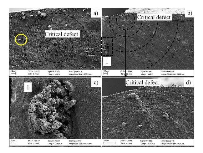
Figure A6: SEM image showing the rupture surface of S\_9.0, a) decohesion at the inclusion, marked by a yellow circle next to the critical defect, b) rupture surface and critical defect (CBaggl) in a material containing ZnO. c) and d) enlarged views of a ZnO inclusion (rectangle 1) and of the critical defect from picture b).
