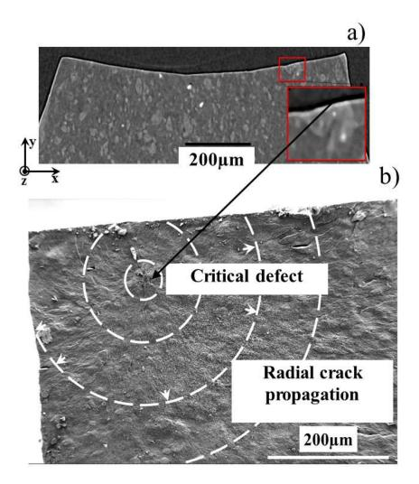
Figure 8: Continuation of Figure 8, a) slice view of the broken sample with the critical defect. The inset photo shows the magnified critical CB<sub>aggl</sub>. B) SEM observation confirming the crack initiation and further propagation of the crack from the critical defect.
