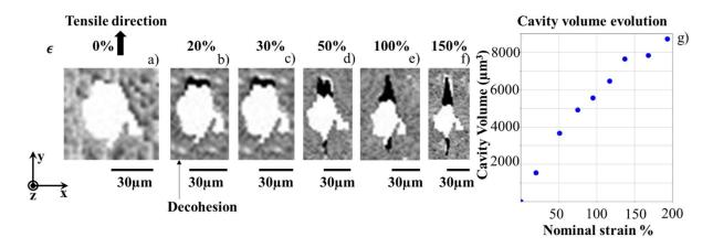
Figure 4: a)-f): damage evolution around a metallic particle with  $V=18000 \mu m^3$  ( $Eq_{diam}=32 \mu m$ ) as a function of deformation: b) decohesion, e) and f) cavity growth in the direction of the applied stress, g) cavity volume around this particle, as a function of nominal strain.
