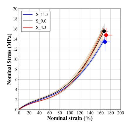
Figure 3: a) nominal stress vs nominal strain for the 3 materials with different concentrations of CB<sub>aggl</sub>. Filled circles (blue: S\_11.5, black: S\_9.0, red: S\_4.3) in the graph denotes the nominal stress and nominal strain at break for the 3 materials.
