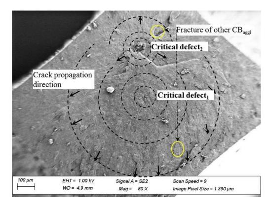
Figure 9: SEM observation of the ruptured surface of S 11.5.
