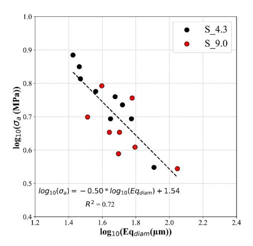
Figure 6: applied true stress at the cavitation onset ( $\sigma_a$ ) as a function of the  $Eq_{diam}$  of the agglomerate in which it occurs (results from S\_4.3 and S\_9.0 materials). Dotted line for the linear curve fitting. Each point in the figure represents an agglomerate either from the material S\_4.3 or S\_9.0 (Note that this already represents a huge amount of work as it requires a careful examination of many images, to avoid any misinterpretation of artifacts).
