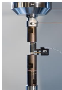
Figure 1. Set-up of cyclic tensile tests.
