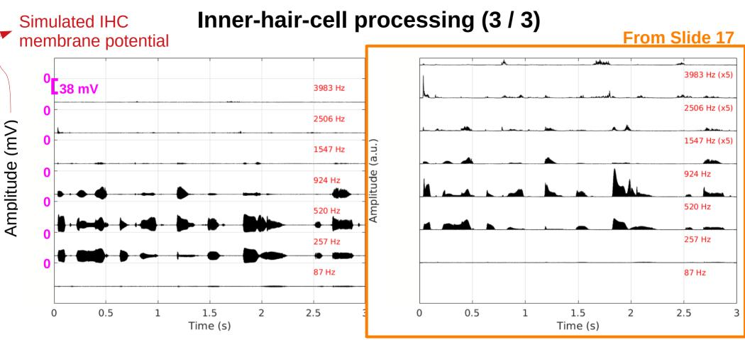
Negative potential (0 V for each channel indicated in magenta) Asymmetric waveforms along V<sub>rest</sub> "Envelope extraction" too for high frequency channels
