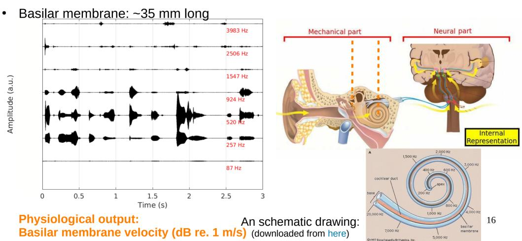
• Typically: Approximated as a half-wave rectification + low-pass filter
