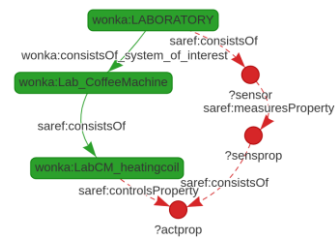
Figure 5: Instantiated query (Req 2.7) with modification proposals to validate the corresponding requirement (green is valid, red is missing, not instantiated and to be added).
