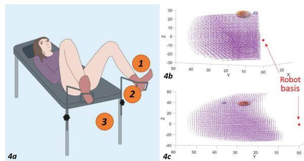
Fig.4: Positions of the robot in relation to the patient during a physical examination [9], modified.
