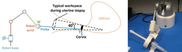
Fig.2: Apollo Robot [5] and its kinematic model.
