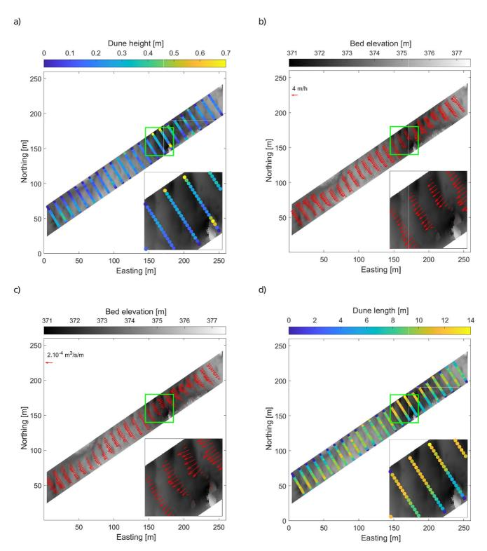
Figure 8. Maps of (a) time-averaged mean bedform height, (b) time-average bedform velocity, and (c) time-averaged bedload rates and (d) time-average bedform length.
