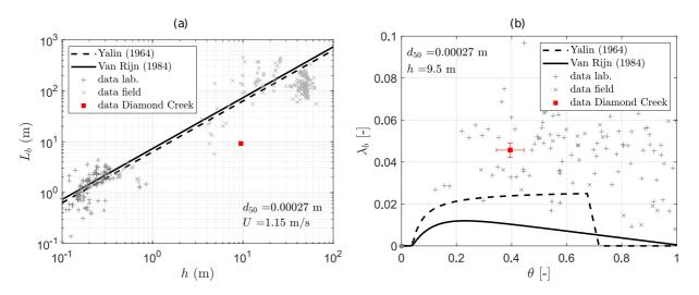
Figure 6. (a) Comparison of observed bedform characteristics and empirical models: bedform wavelength  $L_b$  versus water depth h and bedform steepness  $\lambda_b$  (b) versus the Shields number  $\theta$ .
