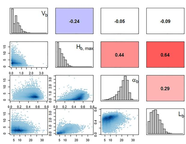
**Figure 5.** Scatterplot and correlation plot (all instantaneous values at all nodes) of dune velocity [m/h], maximal dune height [m], shape factor [-] and dune length [m]. The values of the axis labels are expressed in m/s for  $V_b$ , in m for  $H_{b,max}$  and  $L_b$ , and without units for  $\alpha_b$ .
