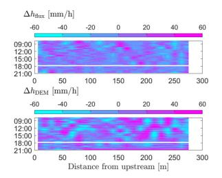
Figure 10. Time-evolution of the computed  $(\Delta h_{\rm flux})$  and observed  $(\Delta h_{\rm DEM})$  bed-evolution rates along the reach.
