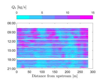
Figure 9. Time-evolution of the instantaneous cross-section-integrated bedload fluxes  $Q_b$  along the reach.
