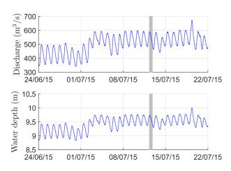
**Figure 2.** Water discharge and mean water depth time series recorded at the U.S. Geological Survey (USGS) Colorado River Above Diamond Creek near Peach Springs, Arizona, 09404200 streamflow gaging station in June-July 2015 (the gray area corresponds to the 12 July 2015 survey).
