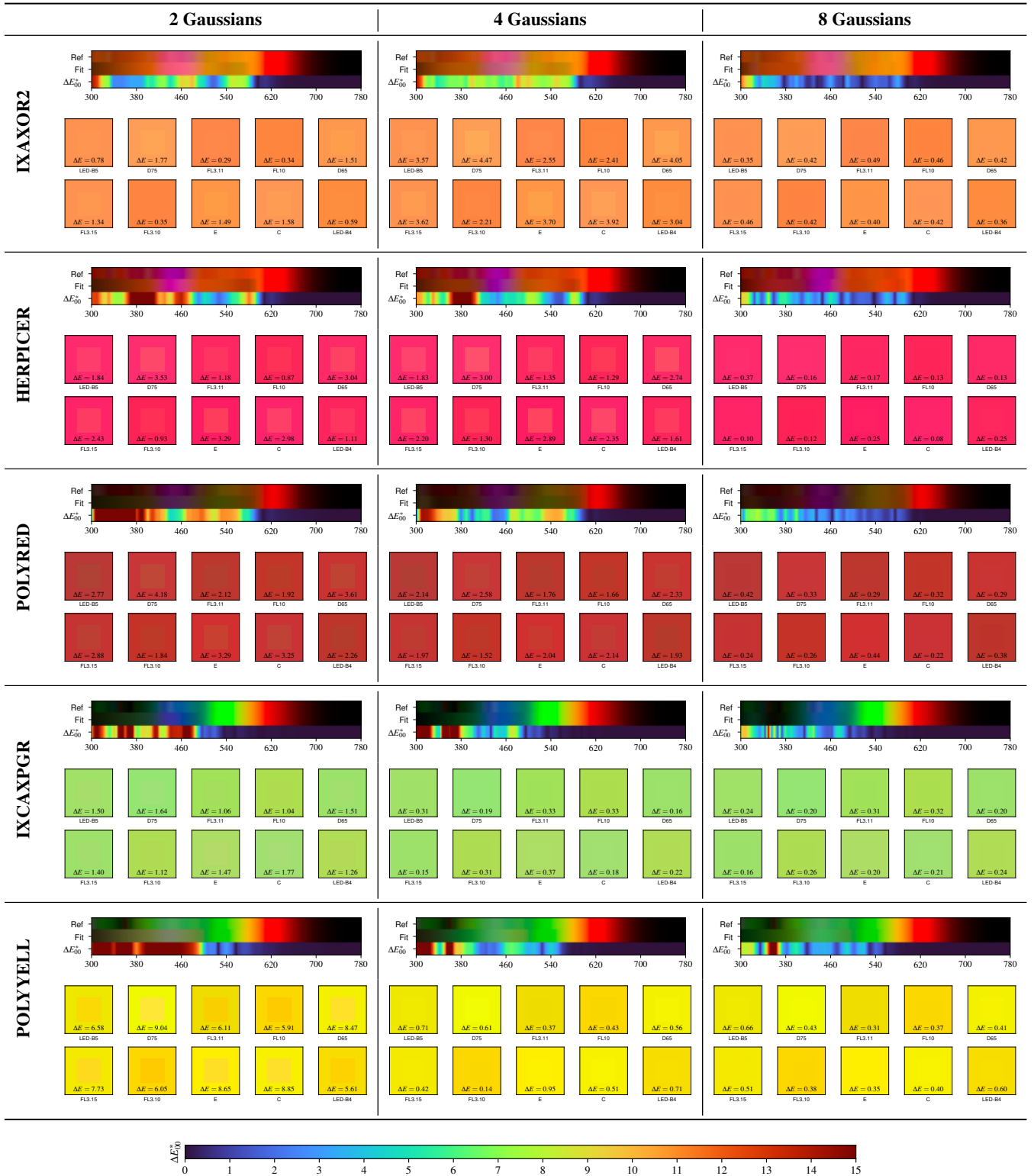
Figure 5: Comparison of analytical renderings based on our fitted model with EM and reradiation matrices. Five worst behaving fluorophores on the fitting of 4 Gaussians based on the average \Delta E_{00}^* over the set of monochromatic illuminants from 300 to 780 nm are showcased. The colour bands show the bispectral reflectance of the reradiation matrix and our corresponding fit under monochromatic illumination along with \Delta E_{00}^* for each wavelength. The colour patches show bispectral reflectance of the fitted model embedded inside of a patch rendered with a reradiation matrix. The worst performing (average \Delta E_{00}^* ) CIE standard illuminants on the whole dataset are displayed.
