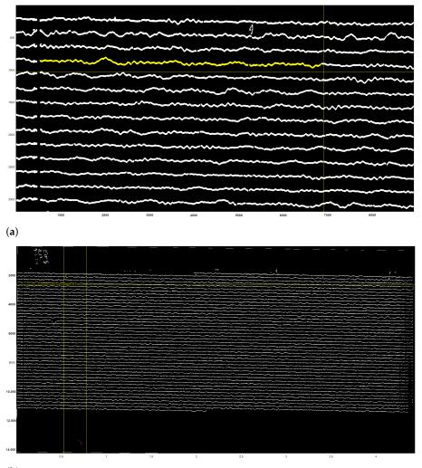
**Figure 11.** Results of the scanned seismogram classification processed by DigitSeis. (**a**) Results of the classified image with shown yellow segments of the identified trace (enlarged fragment). Here: example of file UCC19540109Gal\_E\_0812.tif. Yellow color signifies a selected segment on the trace line.(**b**) Classified seismogram with traces saved in binary format 0–1. Here: example of file UCC19540109Gal\_E\_0812.tif (seismogram recorded on 9 January 1954).
