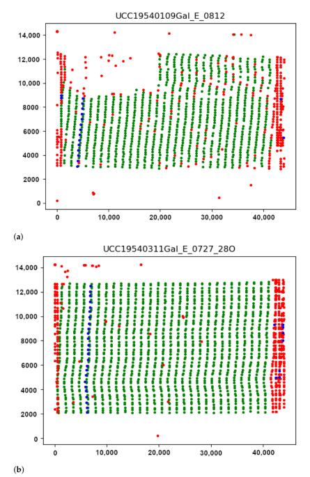
**Figure 20.** Controlling digitising results using Python (Matplotlib library). (a) Quality control for time gaps: missed marks in unrecognised segments. (b) Correctly identified time gaps controlled by Python's Matplotlib. Different color dots are used to separate minute marks (green), hour marks (blue) and margin values and outliers (red).
