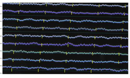
Figure 16. Corrected digitised traces upon completion of the semi-automated vectorisation.(a) Corrected digitised traces upon the completion of the semi-automated vectorisation process.(b) Visible SDT lines (bold) after the semi-automated vectorisation.
