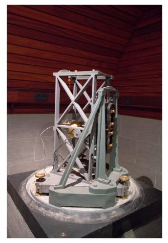
**Figure 2.** Instrument used for data capture in 1954: Horizontal Galitzine seismometer located in UCC. Image source: courtesy of ROB. Photo source: R. S. M. De Plaen.
