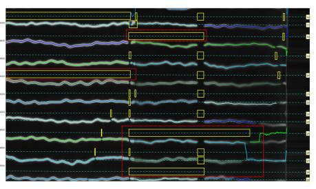
**Figure 13.** Identified traces for selective correction and re-digitising using Correct Trace mode. (a) Identified wrong vector direction of line crossing individual traces. (b) Detected misclassifications caused erroneous digitising. The gaps on the zero-lines (small yellow boxes) show the gaps that existed in the old paper in the original image itself. Differently colored lines are used to distinguish the segments of the traces.
