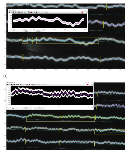
**Figure 15.** Correcting trace for the selected segments. (a) Merging the trace initially broken into the three separate parts (three small yellow boxes). (b) Reclassification of the selected segment and digitising the centroid of the trace line.
