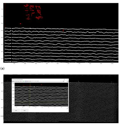
**Figure 10.** Results of the paper seismogram classification processed by DigitSeis. (**a**) Results of the classified seismogram with shown identified object categories (fragment): traces (white) and noise (red, here: handwritten annotations). (**b**) Small region analysis used for defining a smaller area of interest for closer examination of a border region of the seismogram.
