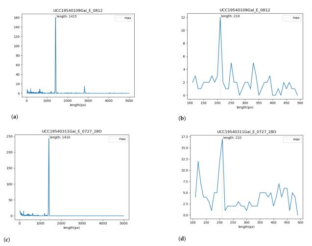
**Figure 21.** Validating the results of segments tracing in Python, Matplotlib for selected seismogram. (**a**,**c**): Frequency of segment length: size of various segments in a trace. (**b**,**d**): Analysis of statistics on segment length per hours of recording. (**a**,**b**): UCC19540109Gal\_E\_0812.mat (**c**,**d**): UCC19540311Gal\_E\_0727\_280.mat.
