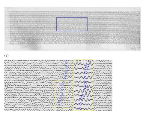
**Figure 7.** Analysing seismogram in paper-based format: traces and time gaps. (**a**) Original scanned seismogram (UCC19540116Gal\_E\_0820.tif). (**b**) Enlarged fragment of image showing time gaps which indicate minute marks and a zoomed segment separating the trace line between each other with tiny white gaps breaking the traces.
