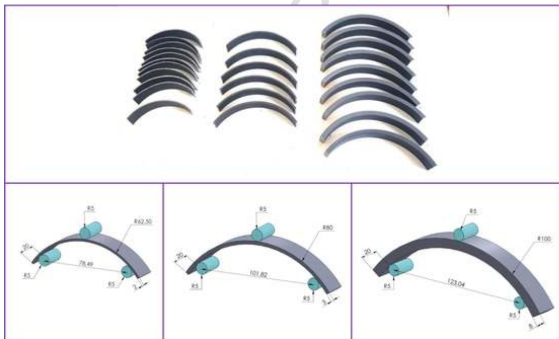
Fig. 2. Extraction and dimensions of curved samples dedicated for curved three point bending (CTPB) tests.
