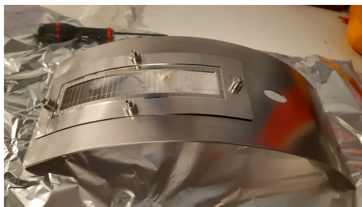
Figure 4. The rectangular hole and grid on the outer curved electrodes of the second version of the spectrometer.
