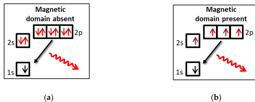
Figure 1. Radiative Deexcitation (a) in the absence of magnetic domains with a fully occupied L-shell and (b) in the presence of magnetic domains with a half occupied L-shell.
