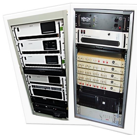
Fig.2 - Equipment set (Double-sided): Model – VIPIR: Vertical Incidence Pulsed Ionospheric Radar Very high interference immunity: IP3 > 45 dBm; High Dynamic Range: 115(I) +30(V) dB; Direct RF sampling 14 bits at 80 MHz; Fully digital conversion, receiver and exciter; Waveform Agility: 2 μs to 2 ms pulse/chip width; USB-2 Data and Command/Control Interfaces; 8 coherent receive channels; Frequency: 0.3 – 26 MHz; 4 kW class AB pulse amplifier; 3rd harmonic < -30 dBc; Precise GPS timing possible for bi-static operation; Radar software Open Source C code; runs under Linux. Courtesy: National Oceanic and Atmospheric Administration – NOAA and National Geophysical Data Center | Terence.Bullet@colorado.edu (2018).
