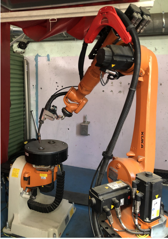
Fig. 17. The system used to manufacture the parts consists in a KUKA robotic arm equipped with a CMT welding torch.
