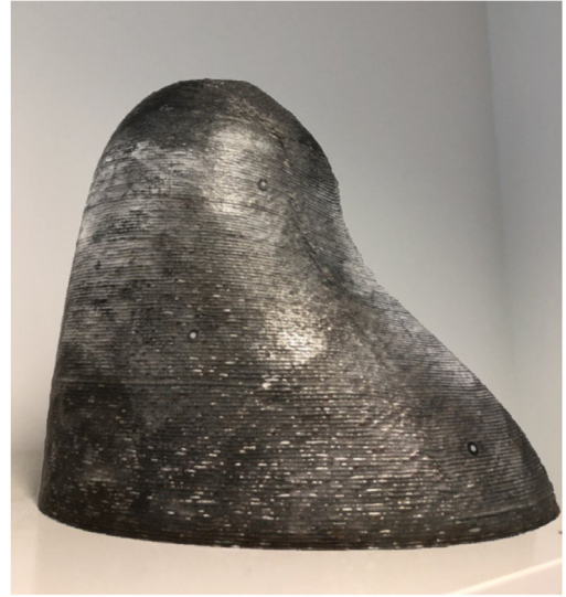
(b) Manufacturing closed part called "Elephant's foot" with an average deposit of 2mm.
