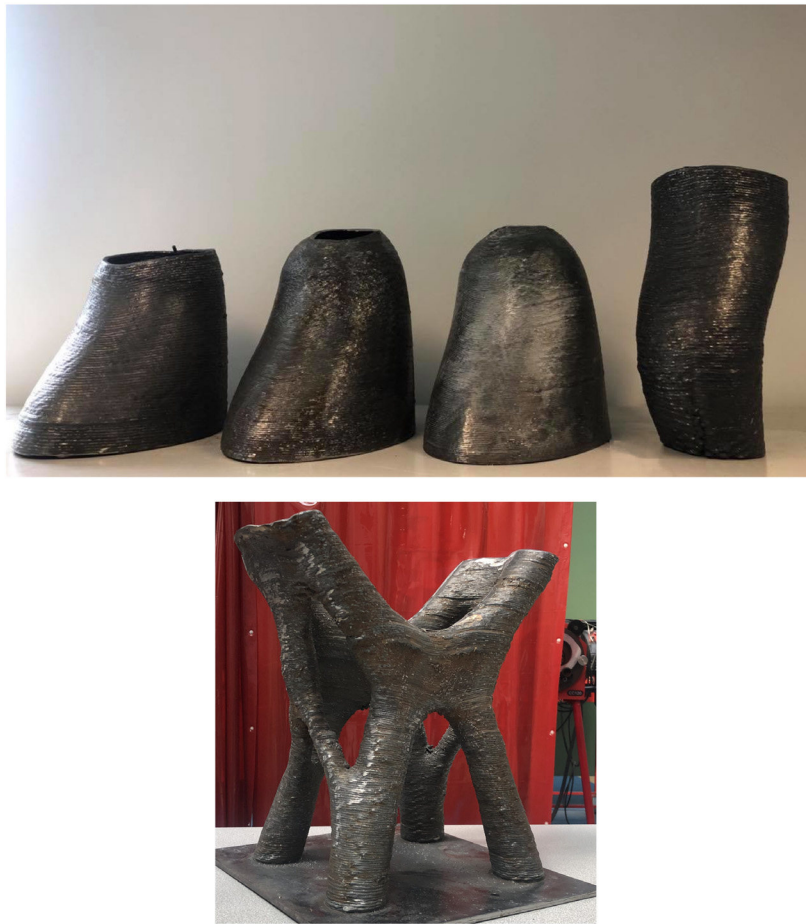
Fig. 21. Three parts manufactured with our Thermal Scalar Field for Continuous Toolpath.
