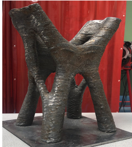
(c) Manufacturing of a multi-branch part from topological optimization with an average deposit of 2mm.
