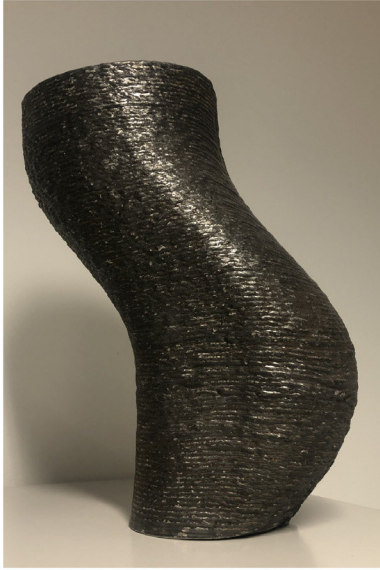
(a) Manufacturing opened part "Elephant's trunk" with an average deposit of 2mm.
