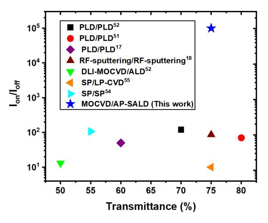
Figure 6. Rectification ratio,  $I_{on}/I_{off}$ , as a function of the average transmittance in the visible for CuCrO<sub>2</sub>/ZnO based heterojunctions, as obtained by literature. Each work is labelled based on the deposition technique used for the CuCrO<sub>2</sub> and ZnO synthesis
