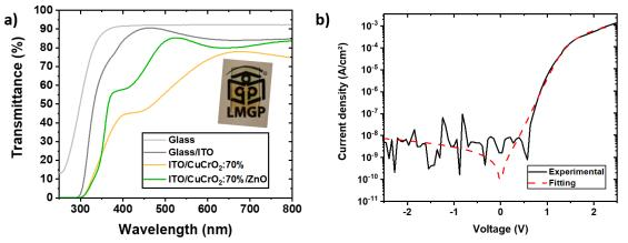
Figure 4. a) Comparison between transmittance spectra of ITO,  $ITO/CuCrO_2$ :70%, and  $ITO/CuCrO_2$ :70%/ZnO. The spectrum of the glass substrate is reported for comparison. The inset shows the macroscopic aspect of the device, before the deposition of the gold contacts. b) Fitting of the  $ITO/CuCrO_2$ :70%/ZnO device characteristics.
