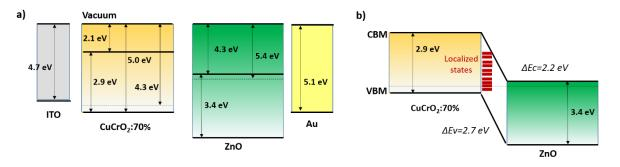
Figure 5. a) Proposed energetic levels of each material prior the contact. The values were obtained by the references and Tauc plot. b) Band diagram for the p-n junction based on CuCrO<sub>2</sub>:70% and ZnO. Here, the interface states are evidenced.
