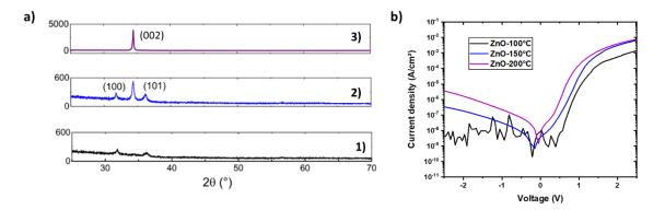
Figure 2. Effect of the deposition temperature of ZnO by AP-SALD a) XRD patterns of the ZnO layers deposited at 1) 100°C, 2) 150°C, and 3) 200°C, adapted by the Nguyen Ph.D. thesis<sup>65</sup>. b) Effect of the deposition temperature of ZnO over the J-V characteristics of the device when combined with CuCrO2:70%. The number of ALD cycles was adapted to obtain a 60 nm film, at each temperature
