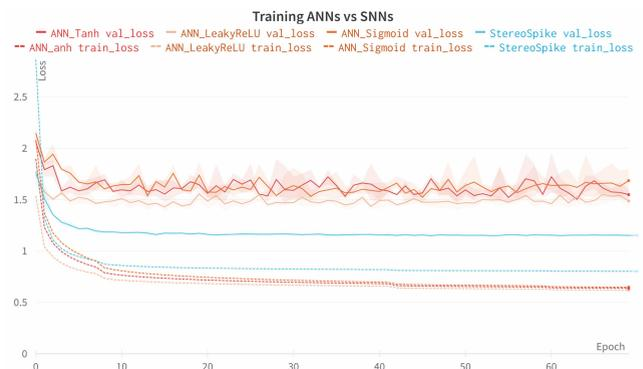
**FIGURE 6.** Learning curves of StereoSpike (blue) compared to equivalent ANN models (orange). StereoSpike’s training and validation loss are respectively higher and lower than their analog relatives by a large margin. This observation is consistent throughout the training procedure and demonstrate the better generalization ability of spiking networks for this task.
