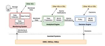
Fig. 2: Closed-control loop components: MS, AE, and DE.
