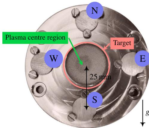
**Fig. 2.** Sintered s.s. target with a pore size of  $5 \mu\text{m}$  after plasma exposure in Magnum-PSI. The discolouration gives a reasonable indication of the central region of the plasma location. The letters in the blue circle indicate the cardinal position of the witness plates, where S is closer to the ground than N. (For interpretation of the references to colour in this figure legend, the reader is referred to the web version of this article.)
