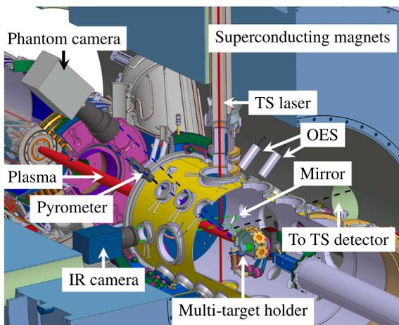
**Fig. 3.** Schematic overview of the relevant diagnostics in Magnum-PSI. The IR camera, the pyrometer, and the OES were all focussed viewing the front centre of the target, while the Phantom camera viewed tangentially to the target.
