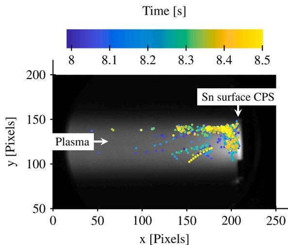
**Fig. 6.** Phantom image of the sintered tungsten target after 8.25 s, overlapping in colour are tin droplets traced using TRACK software at a certain time between 8 and 8.5 s. Droplets shows around  $y \sim 150$  Pixels and  $x > 150$  Pixels are mainly false positives. (For interpretation of the references to colour in this figure legend, the reader is referred to the web version of this article.)
