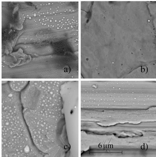
**Fig. 5.** Microscopic image from the WPs to the west of the targets. With (a) the s.s. 100  $\mu\text{m}$  after the last series, (b) sintered W disc, (c) 3D-printed, (d) Felt. The brighter dots are Sn droplets, ranging from nano size covering s.s. 100  $\mu\text{m}$  to the big drop on the right of the 3D-printed target. Sn droplets appear only occasionally for the sintered W disc. Observations of the SEM are inline with the RBS data shown in Fig. 4 and Table 3.
