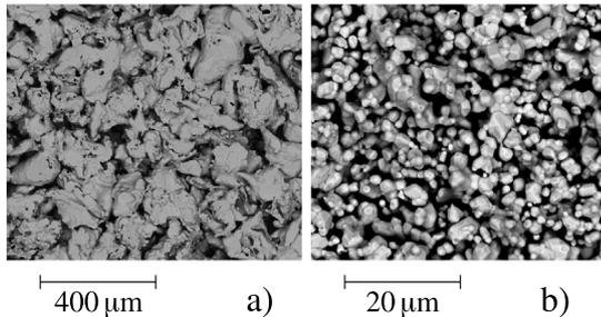
**Fig. 1.** SEM images of the (a) sintered s.s. target with a pore size of 5  $\mu\text{m}$  and (b) sintered W disc. In the W disc the individual powder particles can be seen, while in the s.s. target the powder has fused into a larger structure.
