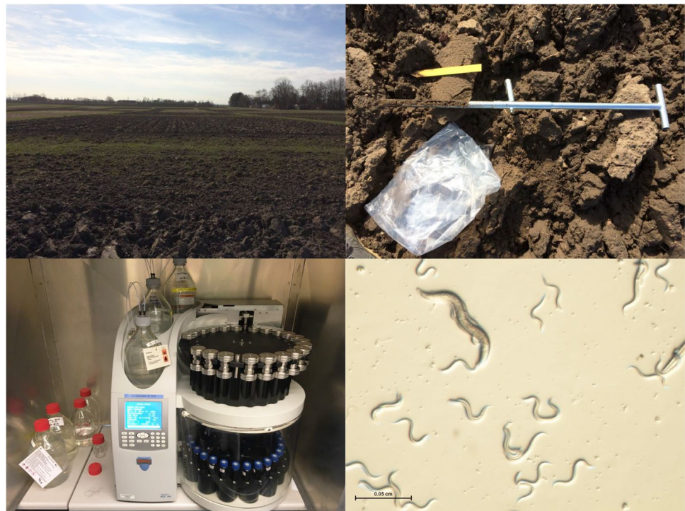
Fig. 1 Upper left: photograph of the CRUCIAL plots, Tåstrup, Denmark; upper right: soil sampling in a CRUCIAL plot; lower left: pressurized liquid extraction with a Dionex ASE 300 accelerated solvent extractor on soil samples collected after waste application; lower right: view of the laboratory nematode species C. elegans under microscope.
