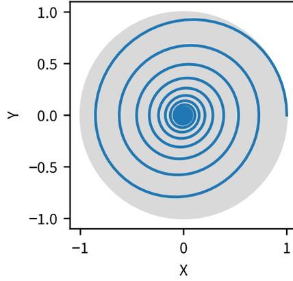
Fig. 16: Trajectory on the equatorial slice of the Bloch sphere of the state of a qubit initialized in the state vector  $|+\rangle$ , evolving under the Hamiltonian  $H = (\omega/2)Z$  and subject to continuous dephasing along the  $X$  axis. Here  $\omega = 1$  and  $\gamma = 0.1$ .
