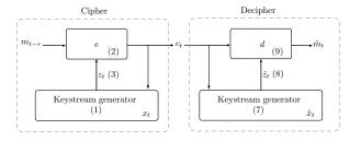
Fig. 1. Self-Synchronizing Stream Cipher block diagram.
