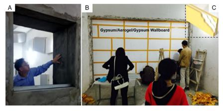
**Figure 15.** Diffuse field sound transmission loss setup preparations. A) View from the connecting window of the test chamber prepared for the 1 m<sup>2</sup> test specimen; B) view from the 10 m<sup>2</sup> aerogel layer; C) schematic for the final configuration of the composite wallboard including two gypsum skin layers accompanied with two core aerogel layers (shown in white).<sup>[105]</sup> (Reprinted with permission.<sup>[105]</sup> Copyright 2018, John Wiley and Sons).
