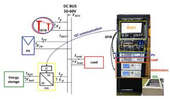
Fig. 3. Experiment platform of the LVDC MG.
