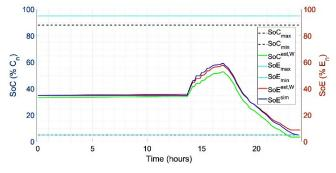
Fig. 8. Comparison of the variations of SoE of 35% between simulation and experimental results relative to SoC limiting values.
