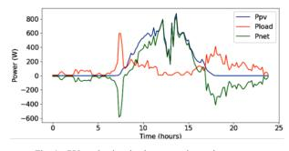
Fig. 4. PV production, load consumption and net power.
