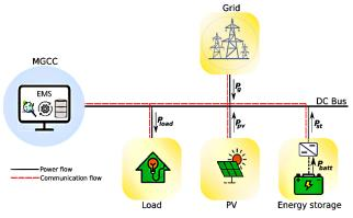
Fig. 2. Grid connected DC MG architecture.
