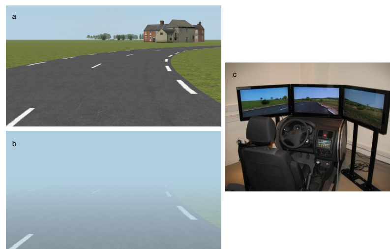
Figure 1. (a) Upper Left: Screenshot of scenario without fog; (b) Lower Left: Screenshot of scenario with fog; (c) Right: Fixed base driving simulator SCANeR.
