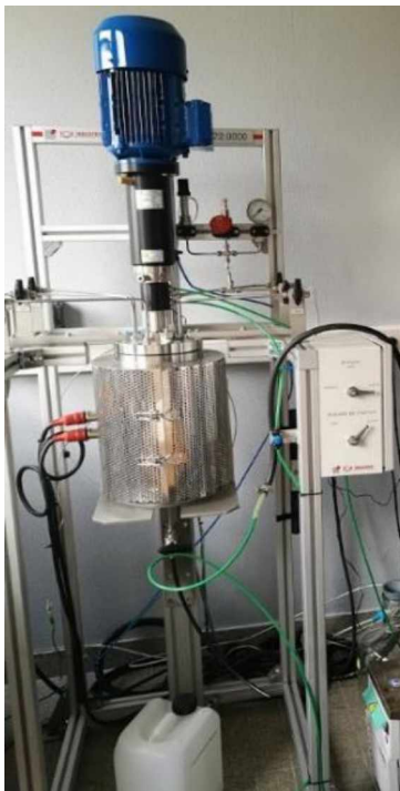
Figure 1. Picture of the 8 L autoclave used for the synthesis of HKUST-1 in which the solution is stirred and thermostated.
