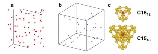
Fig. 1. MD cells containing a) <110> dumbbell SIAs, b) C15 clusters composed of 48 atoms (C15 $_{48}$ ), c) C15 $_{12}$  and C15 $_{48}$  clusters (the orange sphere represents the central bcc atom). Concentration of extraatoms in the cells is  $\sim$ 0.02 %.
