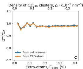
Fig. 6. Relaxation volume per extra-atom for a) dumbbell SIAs, b)  $C15_{12}$  and c)  $C15_{48}$  clusters as a function of extra-atom concentration ( $C_{\text{extra}}$ ) and density of defects  $(\rho_l)$ .  $\Omega^{\text{rel}}$  is given in atomic volume unit  $(\Omega_0)$ .
