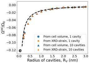
Fig. 9. Relaxation volume per vacant site for a) single vacancies, b) 1 cavity of varying radius, c) 10 cavities of varying radius, d) varying number of cavities of radius 1 nm, e) both 1 and 10 cavities of varying radius as a function of vacant site concentration ( $C_{vacant}$ ) and either radius ( $R_v$ ) or density ( $\rho_v$ ) of cavities. Dashed lines correspond to the predicted relaxation volume computed with  $E_q$ . (7).  $\Omega^{rel}$  is given in atomic volume unit ( $\Omega_0$ ).
