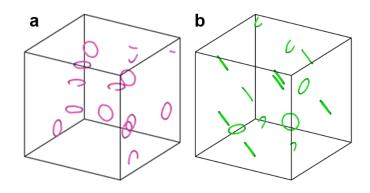
Fig. 2. MD cells containing 12 prismatic a) <100>, b) ½<111> dislocation loops with randomly oriented Burgers vector.
