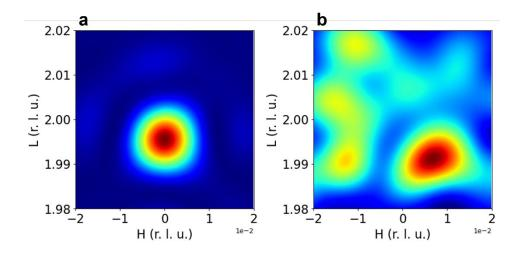
Fig. 4. Computed 002 XRD-RSM of a MD cell containing a) 36 < 100 > dislocation loops of radius 6 u.c., b)  $20 \ 1/2 < 111 >$  dislocation loops of radius 12 u.c.
