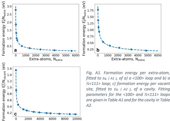
fitted to Eq. (A1), of a) a <100> loop and b) a 1/2<111> loop; c) formation energy per vacant site, fitted to Eq. ( A2 ), of a cavity. Fitting parameters for the <100> and ½<111> loops are given in Table A1 and for the cavity in Table A2.
