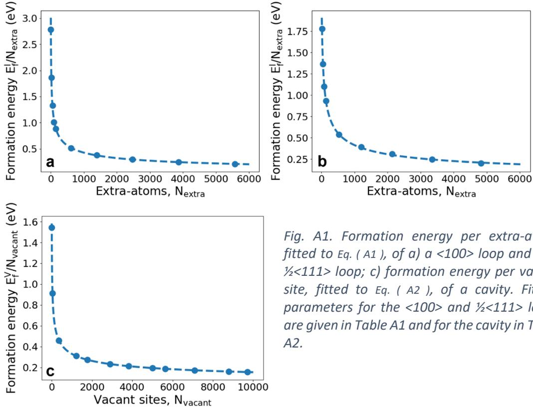
Fig. A1. Formation energy per extra-atom, fitted to Eq. ( A1 ), of a) a <100> loop and b) a  $\frac{1}{2}$ <111> loop; c) formation energy per vacant site, fitted to Eq. ( A2 ), of a cavity. Fitting parameters for the <100> and  $\frac{1}{2}$ <111> loops are given in Table A1 and for the cavity in Table A2.
