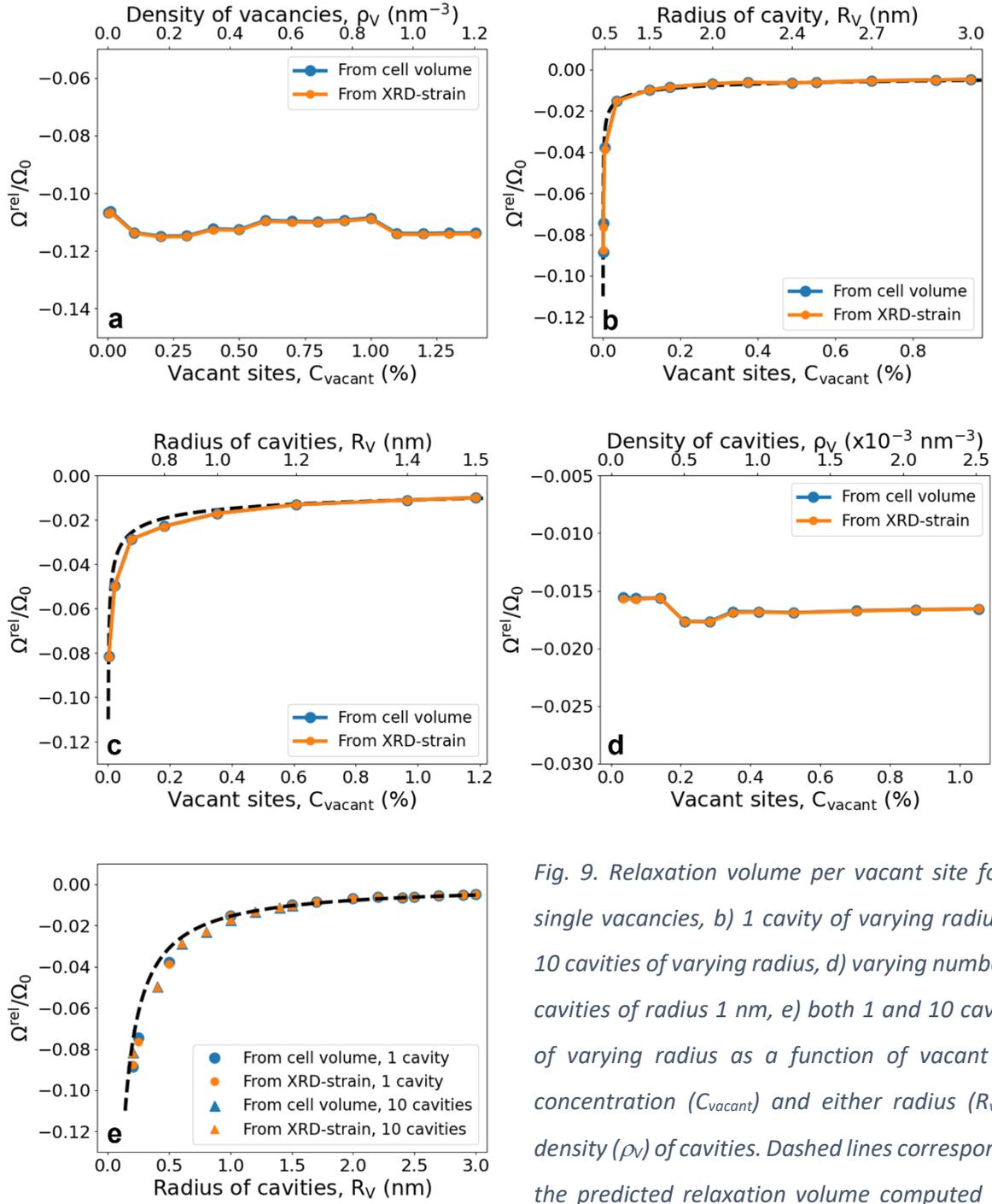
Fig. 9. Relaxation volume per vacant site for a) single vacancies, b) 1 cavity of varying radius, c) 10 cavities of varying radius, d) varying number of cavities of radius 1 nm, e) both 1 and 10 cavities of varying radius as a function of vacant site concentration ( $C_{vacant}$ ) and either radius ( $R_v$ ) or density ( $\rho_v$ ) of cavities. Dashed lines correspond to the predicted relaxation volume computed with Eq. (7).  $\Omega^{rel}$  is given in atomic volume unit ( $\Omega_0$ ).
