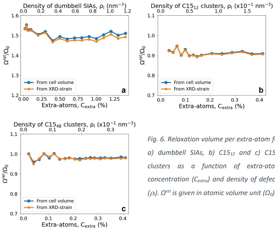
Fig. 6. Relaxation volume per extra-atom for a) dumbbell SIAs, b)  $C15_{12}$  and c)  $C15_{48}$  clusters as a function of extra-atom concentration ( $C_{extra}$ ) and density of defects ( $\rho_i$ ).  $\Omega^{rel}$  is given in atomic volume unit ( $\Omega_0$ ).
