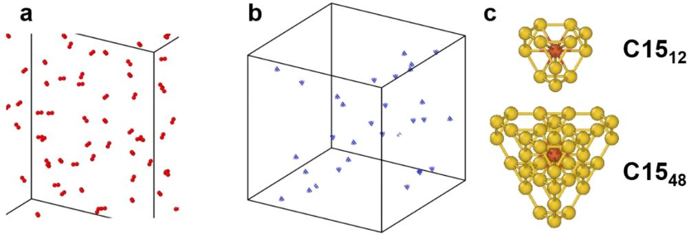
Fig. 1. MD cells containing a)  $\langle 110 \rangle$  dumbbell SIAs, b) C15 clusters composed of 48 atoms ( $C15_{48}$ ), c)  $C15_{12}$  and  $C15_{48}$  clusters (the orange sphere represents the central bcc atom). Concentration of extra-atoms in the cells is  $\sim 0.02\%$ .
