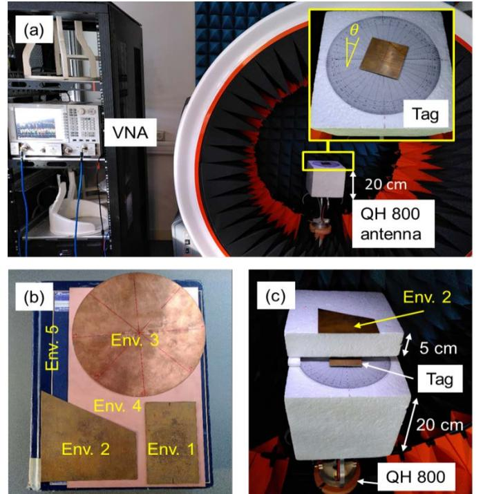
Fig. 3. (a) Picture of the measurement setup. Monostatic measurement in semi-anechoic environment. (b) Different surrounding scatterers used for environment. The scatterers are numbered by increasing RCS level. (c) Surrounding scatterer positioned 5 cm behind the tag.
