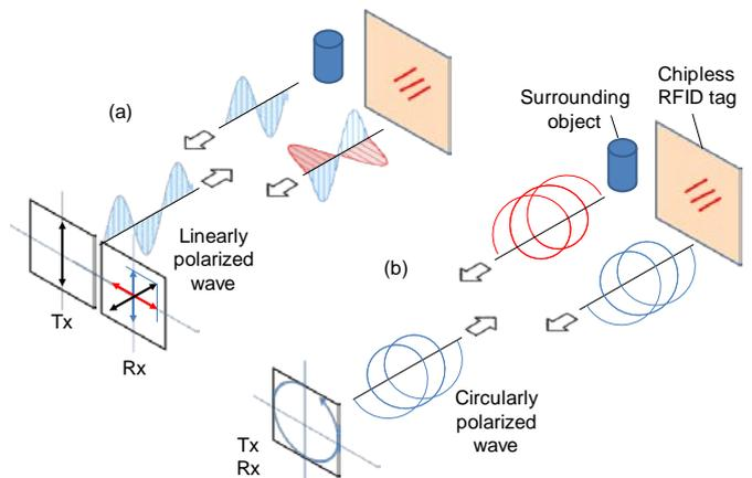
Fig. 1. (a) Cross-polarization interrogation technique [1]. The PSM of the tag has a non-zero cross-component  $S_{vh}$ , which is not the case for classical objects. (b) Circular polarization approach [2-3]. The PSM of the tag has a non-zero component with same handedness (e.g.  $S_{ll}$ ), which is not the case for classical objects.
