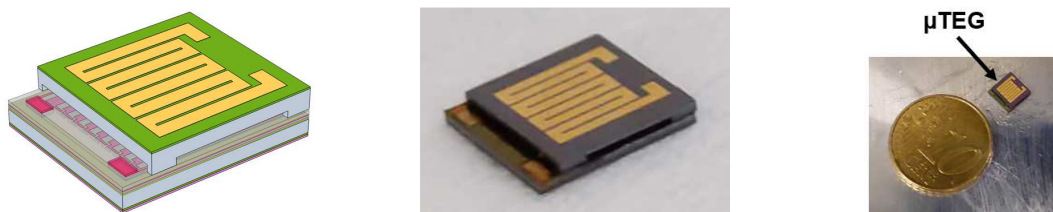
Fig. 10 : Final images of the \mu\text{TEG} after assembly of the concentrator and the suspended membranes.
