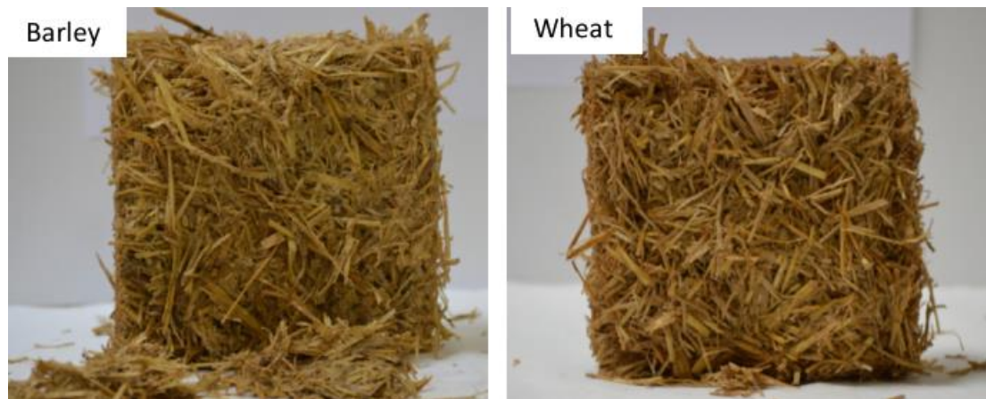
Fig. 9. State of barley and wheat straw composites after 35 and 40 drying-wetting cycles respectively
