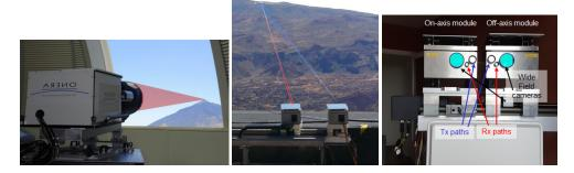
**Fig. 2.** On the left: the GTB, inside the dome of ESA OGS. In the middle: the STB, at the Teide cable car station. On the right, a face view of the STB, showing close-ups of the on-axis and off-axis modules. The downlink beam is in blue, while the uplink beam is in red.
