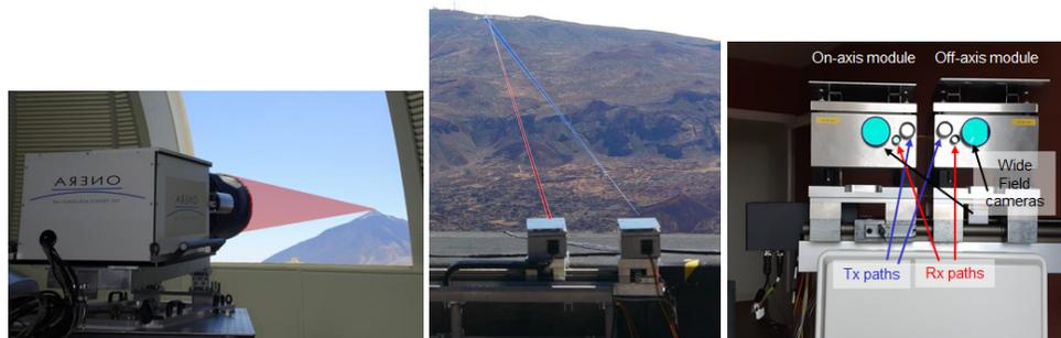
**Fig. 2.** On the left: the GTB, inside the dome of ESA OGS. In the middle: the STB, at the Teide cable car station. On the right, a face view of the STB, showing close-ups of the on-axis and off-axis modules. The downlink beam is in blue, while the uplink beam is in red.
