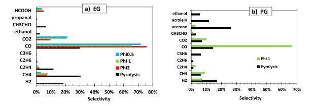
Figure 5: Reaction product selectivity analysis for EG (a) and PG (b) pyrolysis and oxidation at 850 K.
