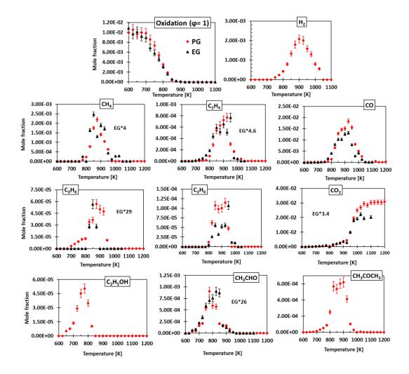
Figure 3: Mole fractions of reactants and main reaction products during the oxidation ( $\varphi = 1$ ) of PG and EG over the temperature range 600-1200 K in the JSR ( $x_{fuel}^{inlet} = 1\%$ , P = 0.107 MPa and  $\tau = 2$  s). Red diamond symbols: PG experiments. Black triangle symbols: EG experiments.
