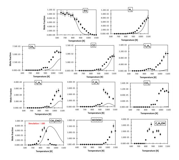
Figure 6: Mole fractions of reactants and main reaction products during the pyrolysis of EG over the temperature range 650-1100 K in the JSR (P = 0.107 MPa and  $\tau = 2$  s). Symbols: experiments. Lines: data computed with the literature model of Kathrotia et al.<sup>8</sup>.
