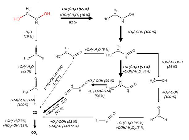
Figure 8: Consumption pathways of ethylene glycol oxidation under stoichiometric condition at 800 K.
