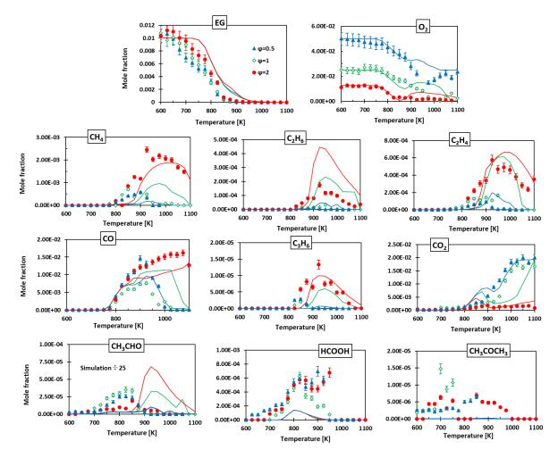
Figure 4: Mole fractions of reactants and main reaction products during the oxidation of 10000 ppm EG in the JSR ( $\varphi = 0.5$ , 1 and 2, P = 0.107 MPa and  $\tau = 2$  s). Symbols: experiments (full triangles:  $\varphi = 0.5$ , empty diamonds:  $\varphi = 1$ , full circles:  $\varphi = 2$ ). Lines: data computed with the literature model of Kathrotia et al.<sup>8</sup>
