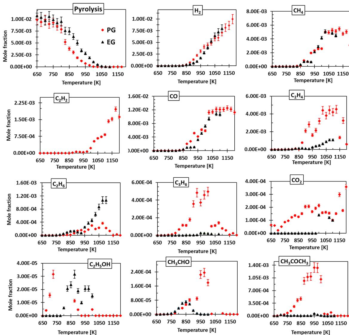
Figure 2: Mole fractions of reactants and main reaction products during the pyrolysis of PG and EG over the temperature range 650-1200 K in the JSR ( $x_{fuel}^{inlet} = 1\%$ ,  $P = 0.107$  MPa and  $\tau = 2$  s). Red diamond symbols: PG experiments. Black triangle symbols: EG experiments.
