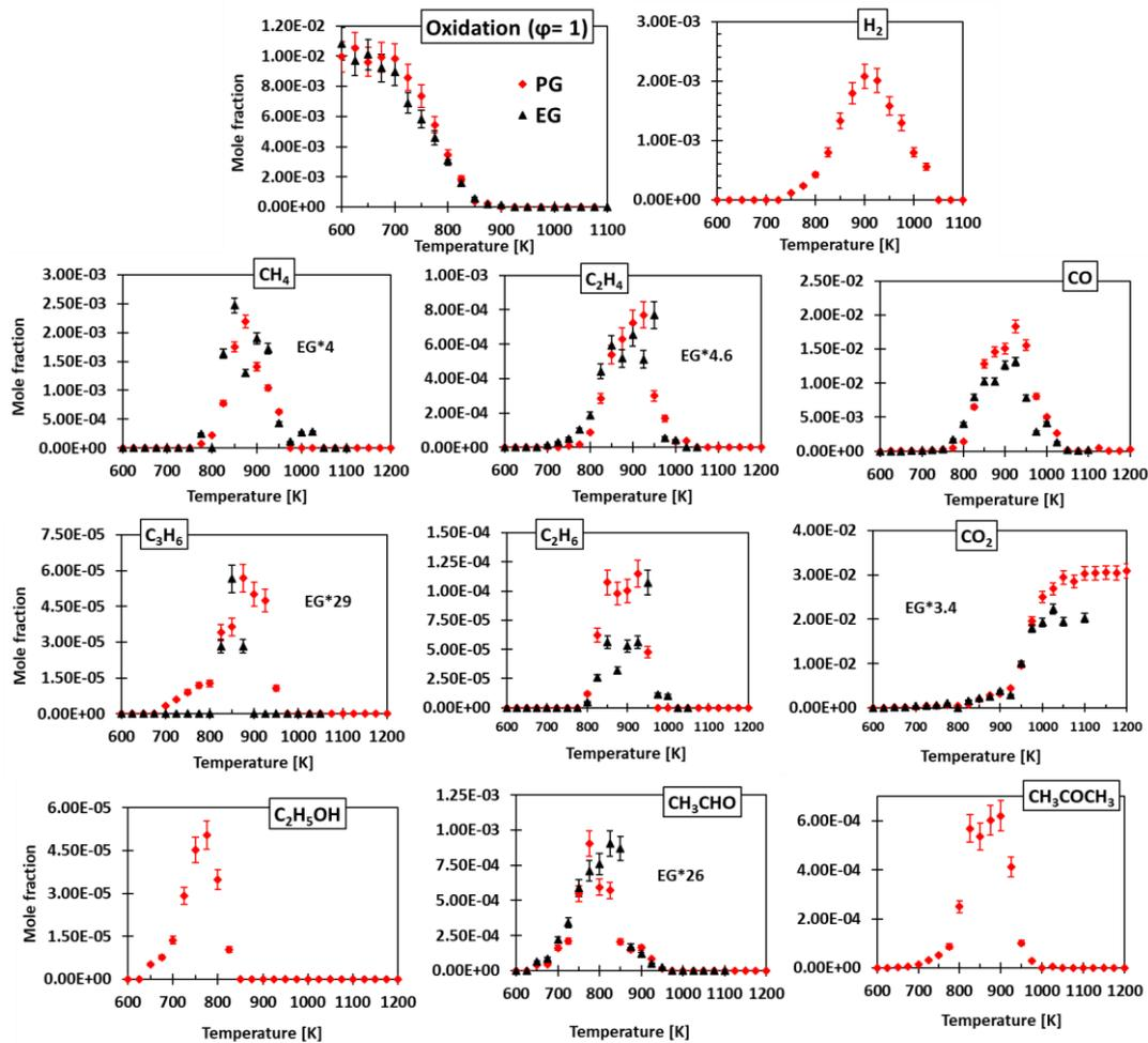
Figure 3: Mole fractions of reactants and main reaction products during the oxidation ( $\phi = 1$ ) of PG and EG over the temperature range 600-1200 K in the JSR ( $x_{fuel}^{inlet} = 1\%$ ,  $P = 0.107$  MPa and  $\tau = 2$  s). Red diamond symbols: PG experiments. Black triangle symbols: EG experiments.
