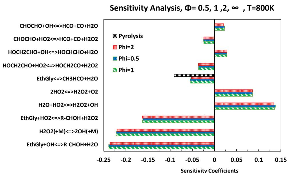
Figure 9: Sensitivity analysis of EG consumption at 800 K for the  $\phi = 0.5, 1.0, 2.0$  (65% fuel conversion) and  $\infty$  (3% fuel conversion),  $P = 0.107$  MPa. A negative sensitivity coefficient stands for a reaction increasing reactivity and vice versa.
