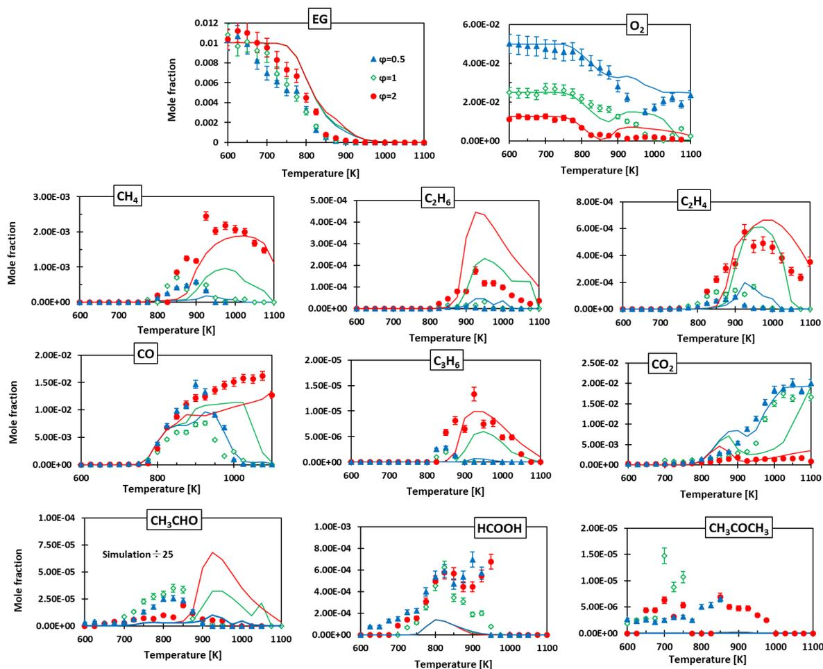
Figure 4: Mole fractions of reactants and main reaction products during the oxidation of 10000 ppm EG in the JSR ( $\phi = 0.5, 1$  and  $2, P = 0.107$  MPa and  $\tau = 2$  s). Symbols: experiments (full triangles:  $\phi = 0.5$ , empty diamonds:  $\phi = 1$ , full circles:  $\phi = 2$ ). Lines: data computed with the literature model of Kathrotia et al.<sup>8</sup>
