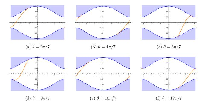
FIG. 1: The bulk and edge state dispersion relations of the Wilson fermion model with  $k_2 = 0$  and m = -1.5 and the boundary condition parameter  $\theta = 2\pi/7$ ,  $4\pi/7$ ,  $6\pi/7$ ,  $8\pi/7$ ,  $10\pi/7$ ,  $12\pi/7$ . The horizontal and vertical axes correspond to  $k_1$  and  $\epsilon$ .
