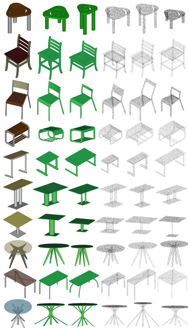
Fig. 8 Generation of as-scanned point clouds for the furniture dataset. First four rows are the chairs (Chair_1 to 4), and next six rows are the tables (Table_1 to 6). First column are CAD templates, second and third are updated meshes, fourth and fifth are virtually-generated point clouds, and last are as-scanned ones
