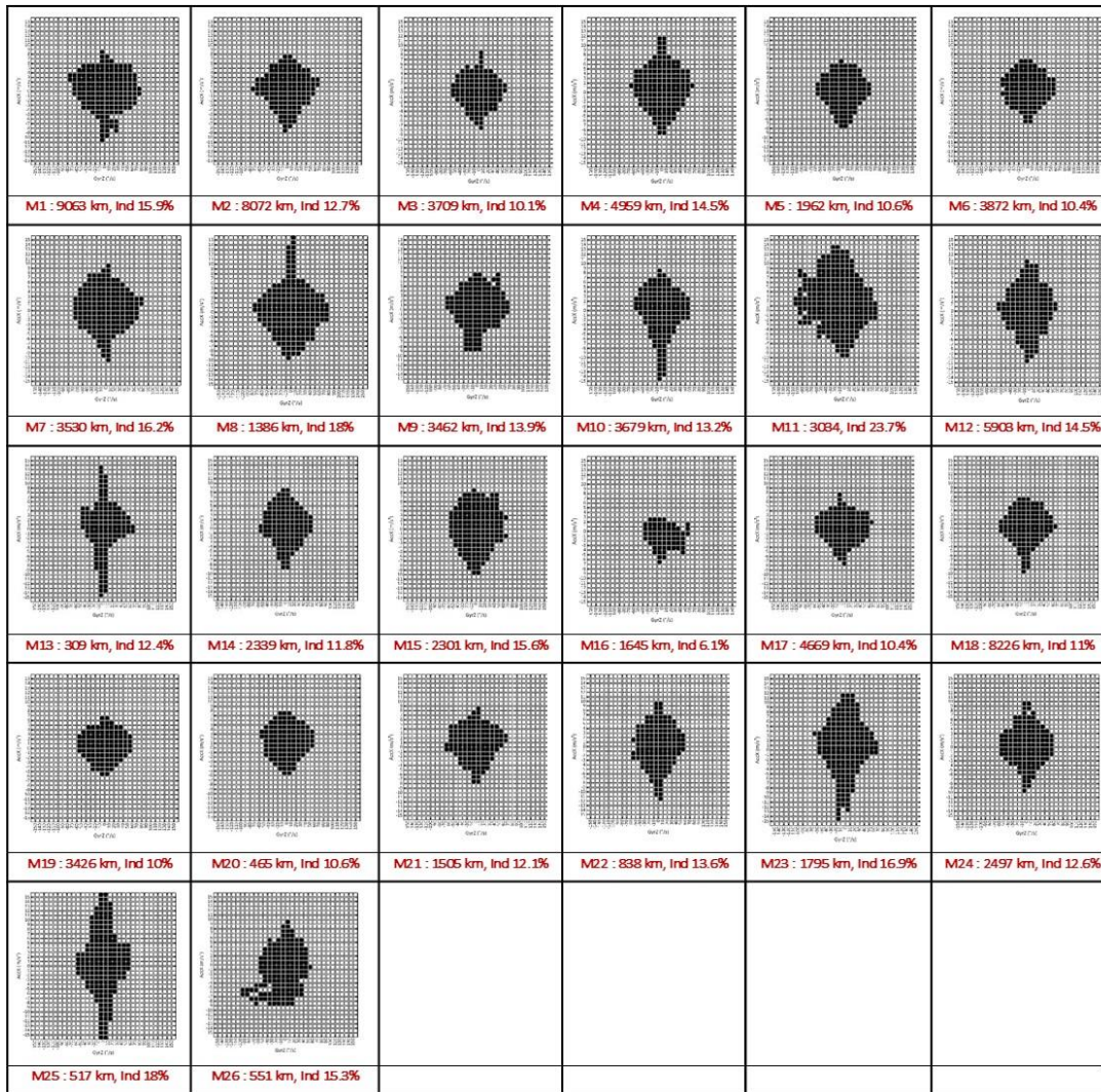
Figure 7: Extreme stress levels of the 26 riders - Longitudinal acceleration vs. Yaw rate
