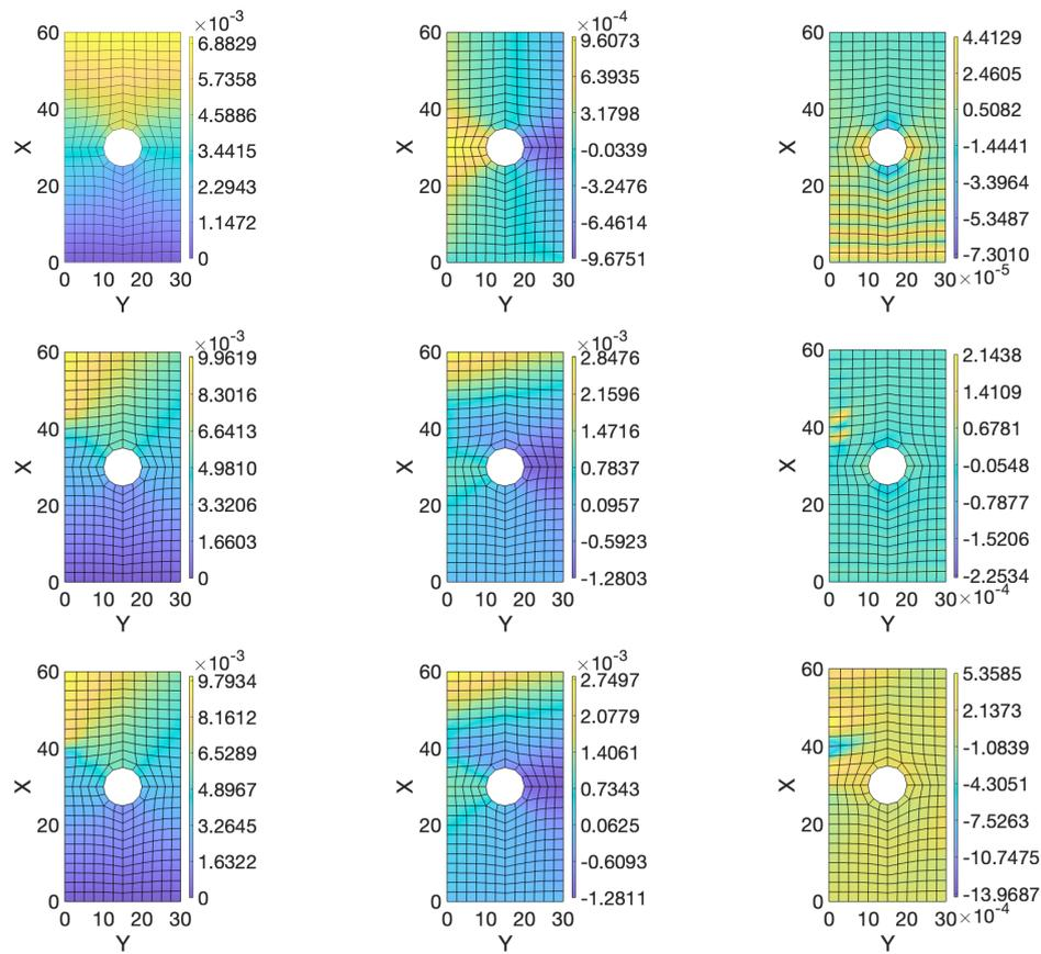
**Figure 11.** Top view of  $x$  (left),  $y$  (center) and  $z$  (right) components of the displacement field associated with the nominal solution (top); reference solution that takes into account the real damaged region (middle) and corrected model solution (bottom).
