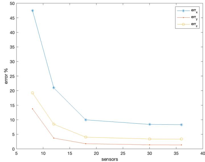
**Figure 22.** Representation of the relative error  $\left( \frac{\|U_{x,y,z}^{Corr} - U_{x,y,z}^{Ref}\|_2}{\|U_{x,y,z}^{Ref}\|_2} \right)$  in percentage, with respect to the number of sensors for the three direction (blue for x-direction, red for y-direction and in yellow for the z-direction). In particular, the result for the 5 different configurations (Figure 21) is specified with some marker and connected with straight lines.
