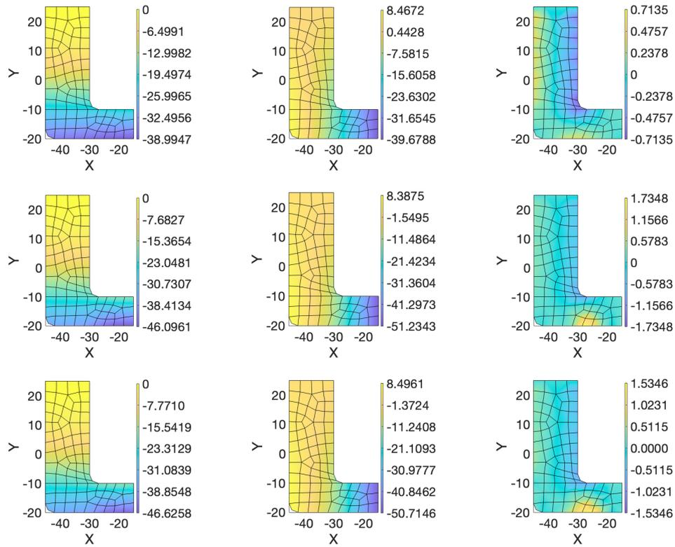
**Figure 16.** Top view of  $x$  (left),  $y$  (center) and  $z$  (right) components of the displacement field associated with the nominal solution (top); reference solution that takes into account the real damaged region (middle) and corrected model solution (bottom).
