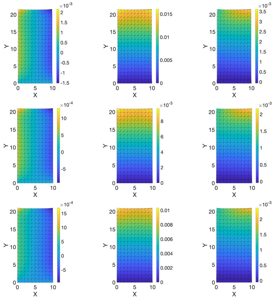
**Figure 19.** Top view of the  $x$  (left),  $y$  (center) and  $z$  (right) components of the displacement field associated to the nominal solution (top), the reference solution (middle) and the enriched model solution (bottom).
