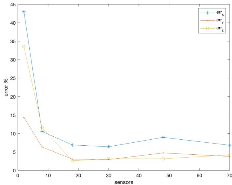
**Figure 7.** Representation of the relative error  $\left(\frac{\|U_{x,y,z}^{Corr} - U_{x,y,z}^{Ref}\|_2}{\|U_{x,y,z}^{Ref}\|_2}\right)$  in percentage, with respect to the number of sensors for the three direction (blue for x-direction, red for y-direction and yellow for the z-direction). In particular, the result for the 6 different configurations (Figure 6) are specified with some marker and connected with straight lines.
