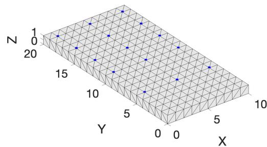
**Figure 18.** Sensors location expected allowing global model enrichment.
