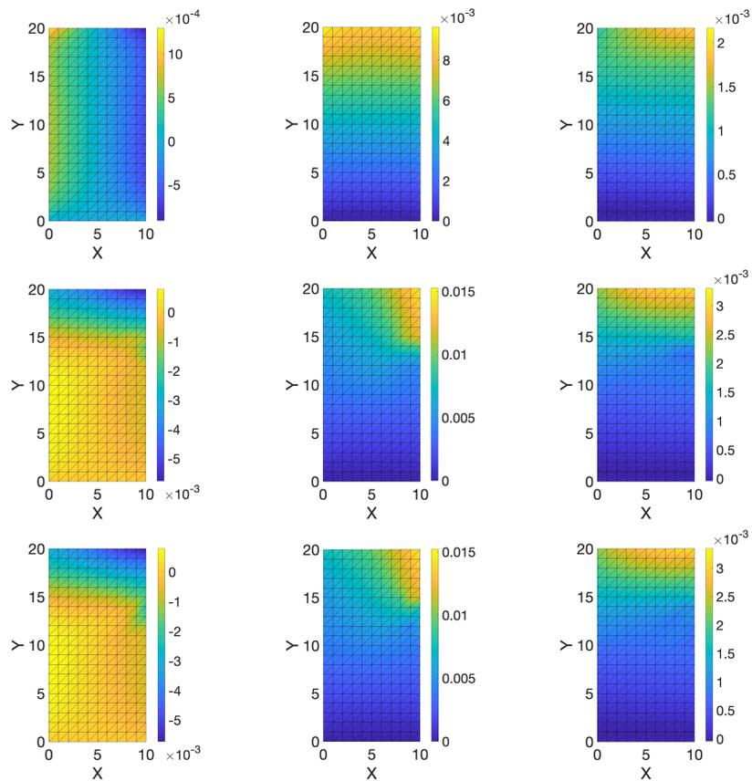
**Figure 4.** Top view of  $x$  (left),  $y$  (center) and  $z$  (right) components of the displacement field associated with the nominal solution (top); reference solution that takes into account the real damaged region (middle) and corrected model solution (bottom).
