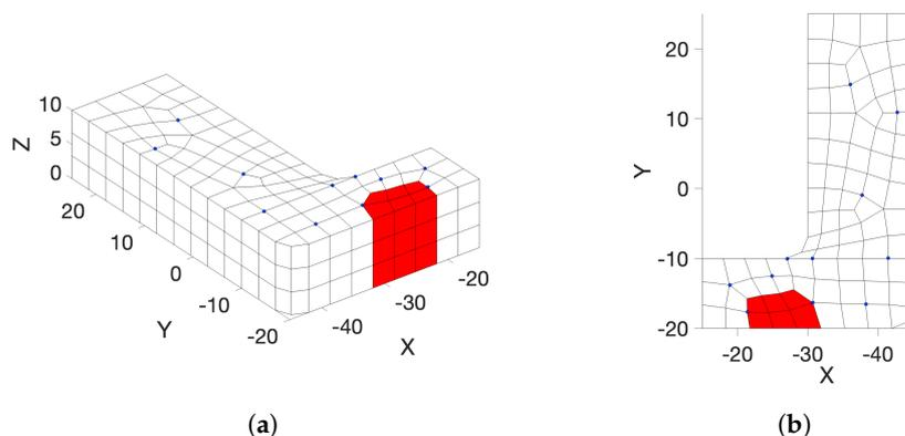
Figure 14. Damaged region (red) and location of the 22 sensors (nodes highlighted in blue). (a) Top view; (b) bottom view.
