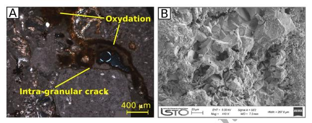
Figure 5. A) SEM observation of micro-porosity in limestone rock from B2 at 9.7 m deep. B) Polarized microscopic observation of calcareous matrix showing oxidation and intra-granular crack, from B2 at 11.1 m deep. Modified from [34].
