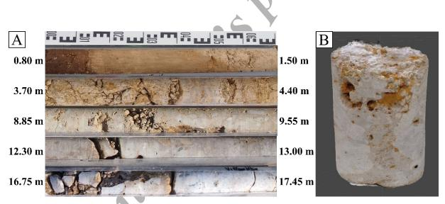
Figure 4. A) Pictures of cores from B1 (70 cm each) taken in the four facies presented in Figure 2. B) 3D reconstruction of a core sample taken from B7 at 11 m deep.
