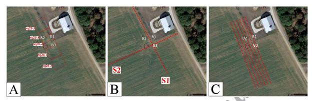
Figure 7. Surface field measurements presented in this study. A) NMR loops of Jan. 2019. B) Seismic lines of Oct. 2018. C) Electric lines of Apr. 2019.
