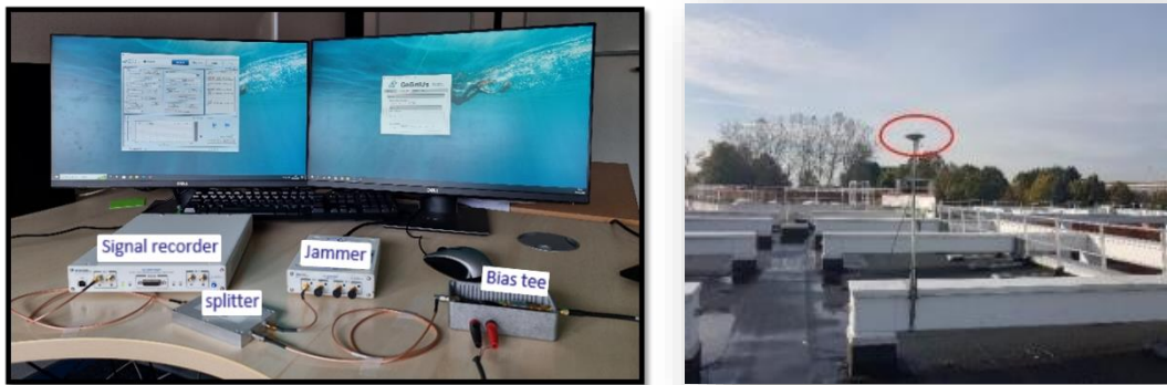
Figure 3 GNSS Signal Recording System Connected to an Interference source (Left) and Antenna The Roof Mounted on The Roof of The Building to Capture Satellite Signals (Right).
