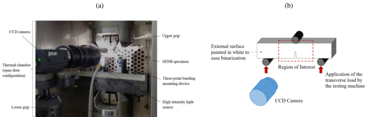
Figure 2 – Monitoring of the crack growth by means of a digital images analysis technique: (a) experimental set-up – (b) schematic representation of the SENB specimen
