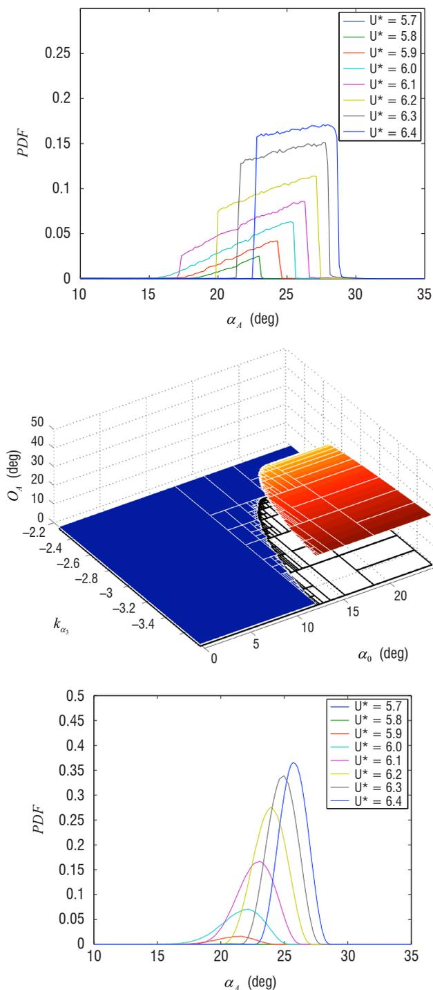
Figure 7 – Up: pdf of the stable large amplitude LCO branch due to uncertainties in  $\alpha(0)$  and  $k_{\alpha_3}$  described by uniform distributions. Mid: corresponding ME-gPC response surface computed for  $U^* = 6$ . Bottom: distribution of  $\alpha_{LCO}$  assuming the  $k_{\alpha_3}$  and  $\alpha(0)$  follow independent  $Beta(\alpha = 3, \beta = 3)$  distributions [52]
