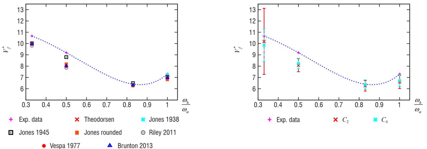
Figure 13 – Linear flutter boundary as a function of the ratio of uncoupled natural frequencies in pitch and plunge. Left: Comparison between experimental data [102] and values of the flutter speed  $V_f^*$  obtained from the approximations of the lift function  $C(k)$  (Table 5). Right: Prior distributions of the model coefficients constructed according to Equation 15 using Monte Carlo sampling with  $10^7$  samples.
