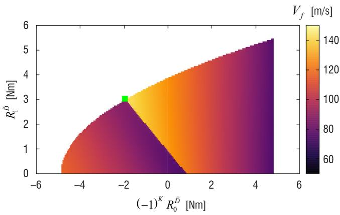
Figure 9 – Response surface of the critical flutter speed  $V_f$  defined in the polar domain for orthotropic laminates [78] for the cantilevered plate wing (Figure 8). The green dot corresponds to the configuration depicted in Table 3 and giving the maximum flutter speed.
