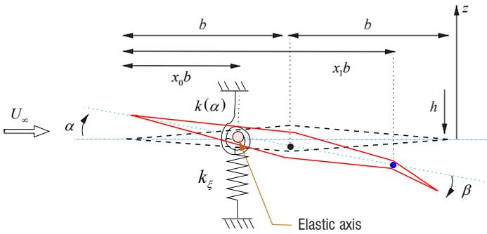
Figure 3 – Two-degree-of-freedom pitch-and-plunge supersonic lifting surface model, with  $b$  the half chord,  $x_\alpha$  the dimensionless static unbalance and  $U_\infty$  the free-stream velocity
