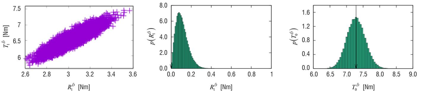
Figure 10 – Scatter plots and distributions of modified bending polar parameters  $R_1^D$  and  $T_0^D$  due to uncertainties in angular ply placement and thickness based on the nominal configuration of the composite laminates in Table 3 [78]
