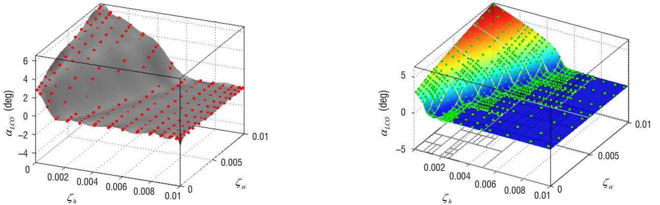
Figure 4 – Left: gPC response surface of  $\alpha_{LCO}$  at  $M = 2.1$  obtained using polynomial order  $P = 14$ . Right: ME-gPC results. The deterministic aeromechanical parameters are [21]:  $x_\alpha = 0.25$ ,  $r_\alpha = 0.5$ ,  $b = 1.5$ ,  $\bar{\omega} = 1$ ,  $\mu = 50$ ,  $x_0 = 0.5$ ,  $\mu = 50$ ,  $\gamma = 1.4$ ,  $B = 5$
