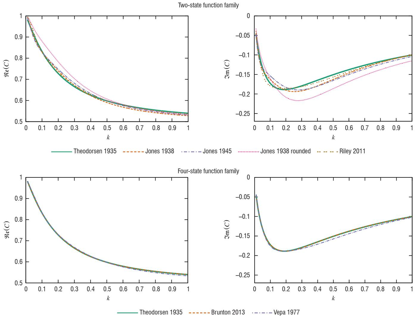
Figure 12 – Plots of typical approximations of the Theodorsen function  $C(k)$  taken from [18, 75, 89] as described in Table 5.
