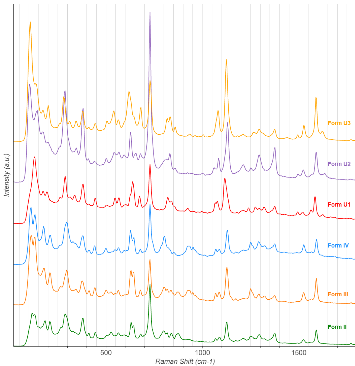
SIF Figure 9: Raman spectra of different crystalline forms of Sulfathiazole, measured on crystals obtained in water droplets with QEPro Raman spectrometer, 785nm.
