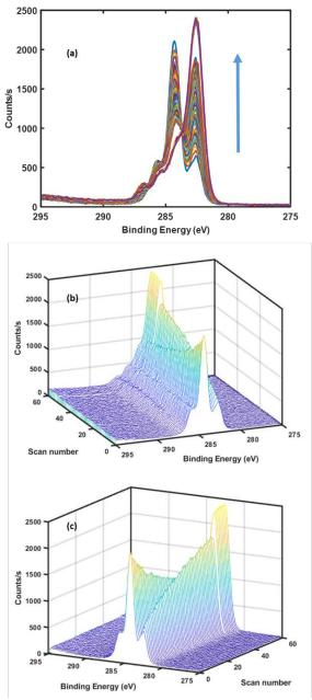
Figure 2. (a) Overlay plot, and (b-c) waterfall plots of 60 C 1s narrow scans from an XPS analysis of cellulose, where (b) and (c) show different views of the same data. The arrow in (a) indicates the order in which the data were collected.
