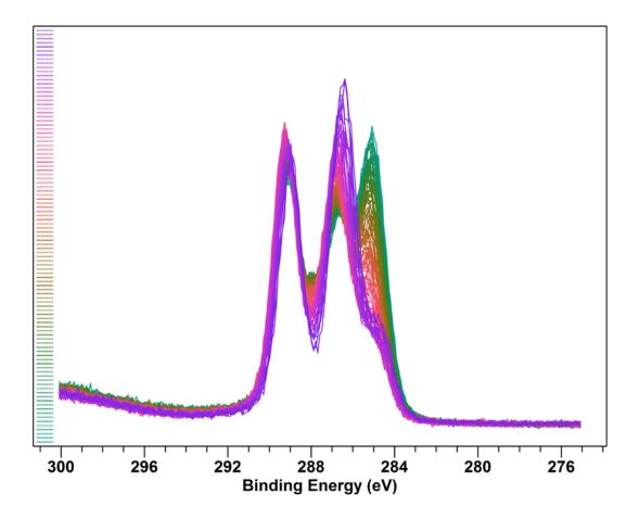
Figure 3. Overlay plot of the C 1s spectra from the tartaric acid data set, where the order in which the spectra were collected is indicated by the colors of the spectra. The scale on the left of the plot indicates that the violet-colored spectra were collected first and the green-colored spectra were collected last.
