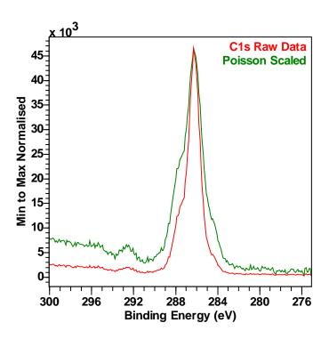
Figure 6. Raw C 1s spectrum of sucrose (red/bottom), and the same spectrum preprocessed by Poisson scaling (green/top). See Section D8 for details on Poisson scaling.
