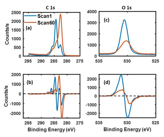
Figure 4. The first and the last (60<sup>th</sup>) undifferentiated (a and c) and differentiated/derivative (b and d) C 1s and O 1s narrow scans of the cellulose data set.
