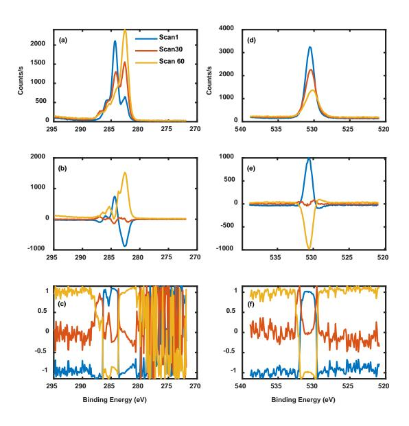
Figure 5. Raw (a) C 1s and (d) O 1s spectra (scans 1, 30, and 60) from the cellulose data set. (b, e) These spectra after mean centering. (c, f) These spectra after autoscaling.
