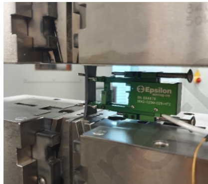
Figure 4. Image of the tensile test setup on the Zwick/Roell Z050 machine displaying the mounted sample and the extensometer.
