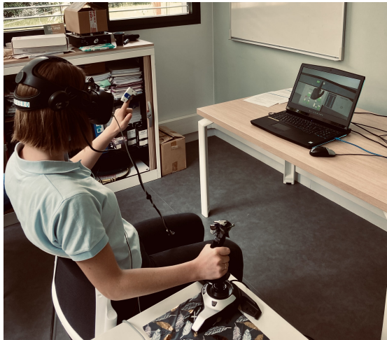
Figure 2: The experimental setup. The participant is wearing an HTC Vive headset equipped with the Leap Motion Controller. In her left hand, she is wearing the Go Touch VR controller. She holds a joystick Cyborg X Flight Stick in her right hand to perform the TRACK task.
